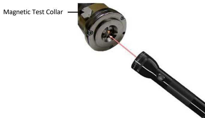
Fig 7-1: Placement of Magnetic Collar and Testing with Test Lamp
