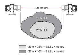
The measurement of combustible gas and air along the optical path length is expressed in LEL• meters, a unit of measurement for the amount of gas present in the length of the light beam.
